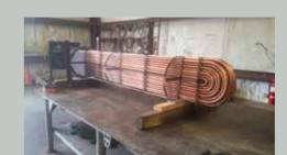
The purpose of refurbishing a heat exchanger is to return it to a standard, equal to, or better than the original specification. This can be performed in a dedicated facility or in the field. Many units have to be re-tubed onsite. It is not unheard of to replace thousands of tubes in excess of thirty feet in length without removing the unit from its place of original field construction. Examples include: turbine condensers, tubular air heaters, and high-pressure water heaters.
